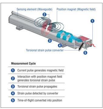
Fig. 1: Time-of-flight based magnetostrictive position sensing principle
