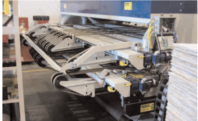
The Accustak is an automated downstacker that can handle 200 sheets/minute with four to eight new setups per shift.
