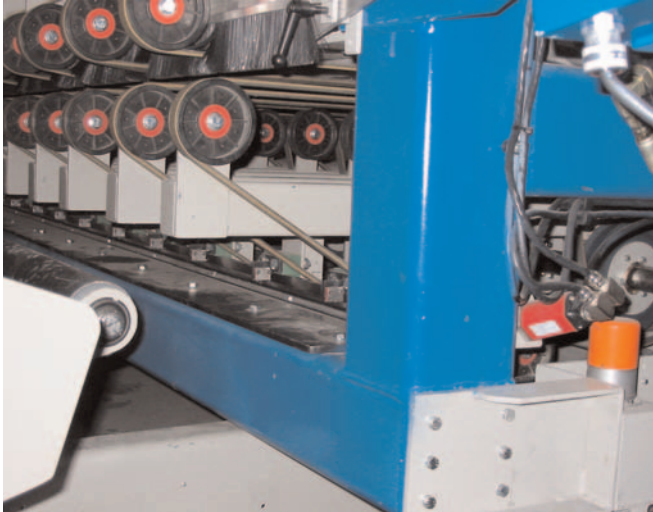
The Accustak automated downstacker with an integrated MTS Temposonics Sensor.
