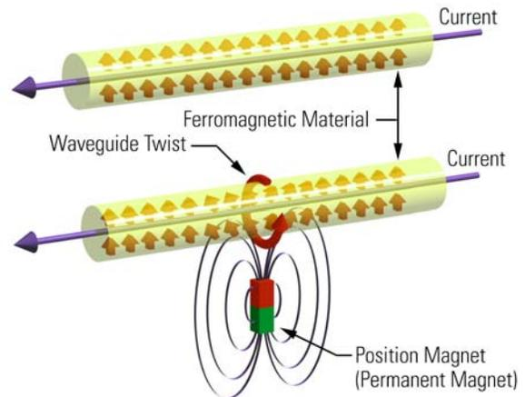
**Figure 7.** Magnetostrictive sensors employ a time-of-flight measurement technique by launching a strain pulse from the moving magnet position that travels at the speed of sound in the Magnetostrictive wire until it is detected by a pickup.
