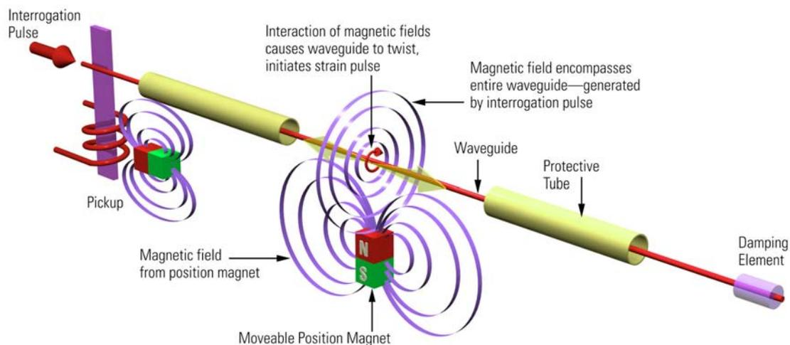
Figure 1. Magnetostrictive Principle
