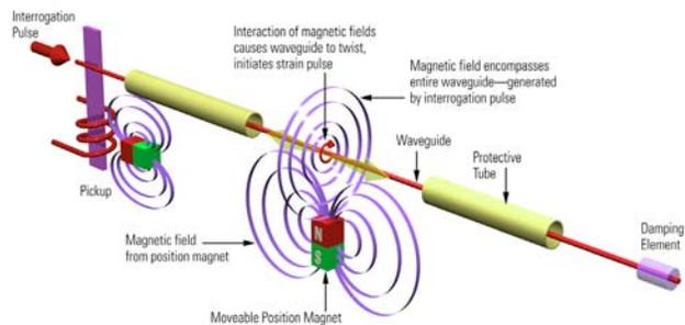
**Figure 8.** The Magnetostrictive Principle.
