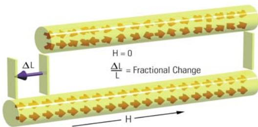
**Figure 6.** Magnetic domains align in ferromagnetic materials when exposed to a magnetic field, causing a dimensional change.
