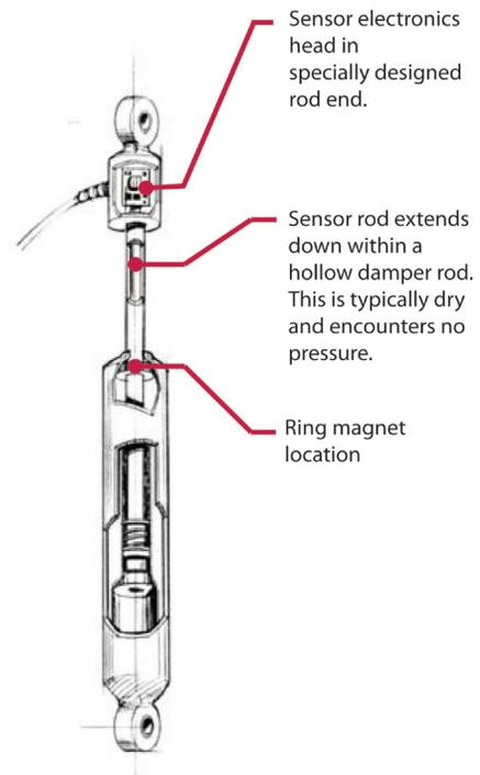
(Fig. 1, Example of a Dry, Rod-End Installation)
