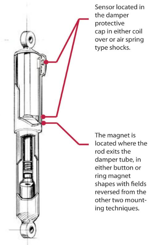
(Fig. 3, Example of a Non-Coaxial Protective Cap Installation)
