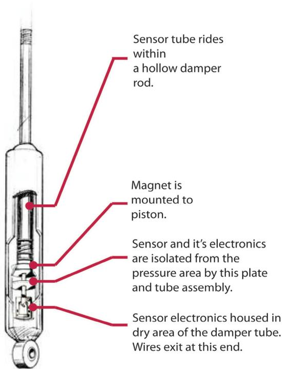
(Fig. 2, Example of a Wet, Tube-End Installation)
