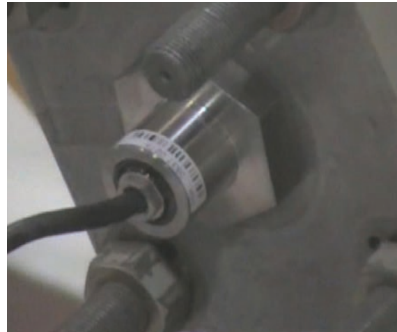
R-Series Model RD4 Sensor rod installed in cylinder end cap with minimal available clearance.
