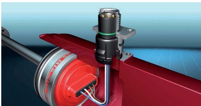
Figure 8. The connector insert is taken out of the cylinder through a bore hole. The flange housing can be snapped into position easily from outside.
